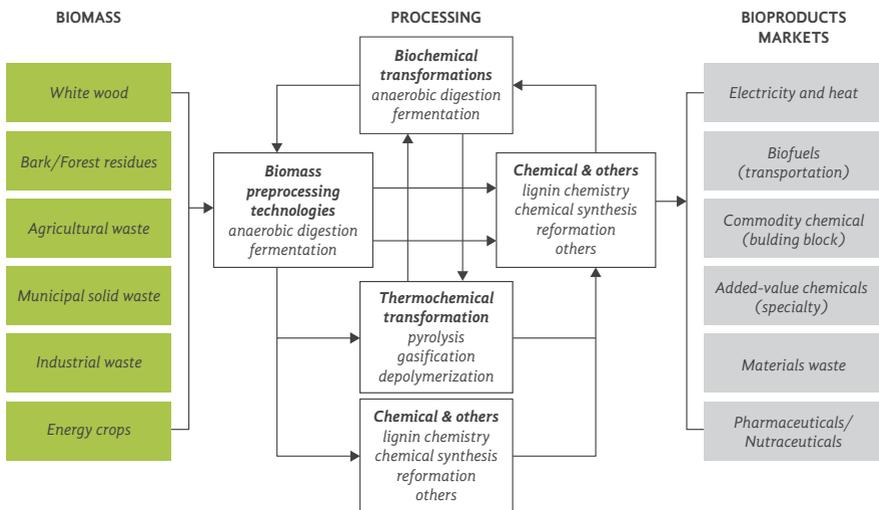
Figure 1. Biorefinery feedstocks (upstream side), conversion technologies and product markets (downstream side). Source: *Systems Perspectives on Biorefineries*, 2013.
