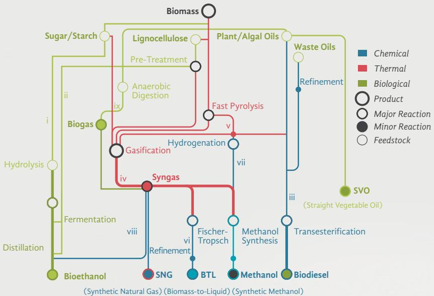
Figure 3. The multiple synthetic conversion routes of major biofuels produced from first and second-generation biomass feedstock. Source: WEC, 2010.
